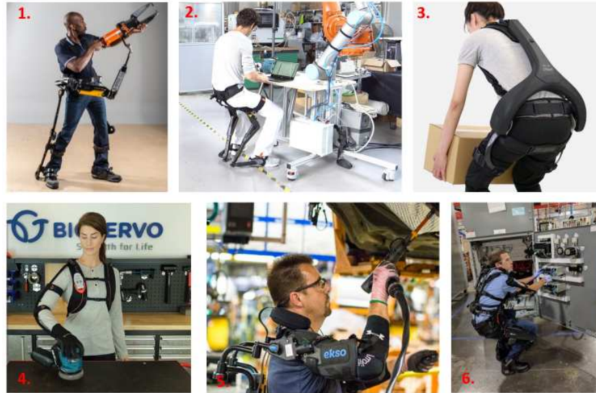
Figure 7.3-2 Exoskeletons for industrial use: 1. Fortis by Lockheed Martin Corporation (courtesy of Lockheed Martin), 2. Noonee “Chairless Chair” (courtesy of Noonee), 3. Powered Wear ATOUN MODEL Y (courtesy of ATOUN), 4. BIOSERVO Ironhand powered glove (courtesy of Bioservo Technologies AB), 5. ©EksoVest by Ekso Bionics upper body exoskeleton, 6. MAX© - Modular Agile eXoskeleton by suitX©.
