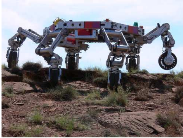
Figure 7.4-4 The robot ATHLETE, climbing a hill with high slope. Image rights: reproduced courtesy NASA/JPL-Caltech.
