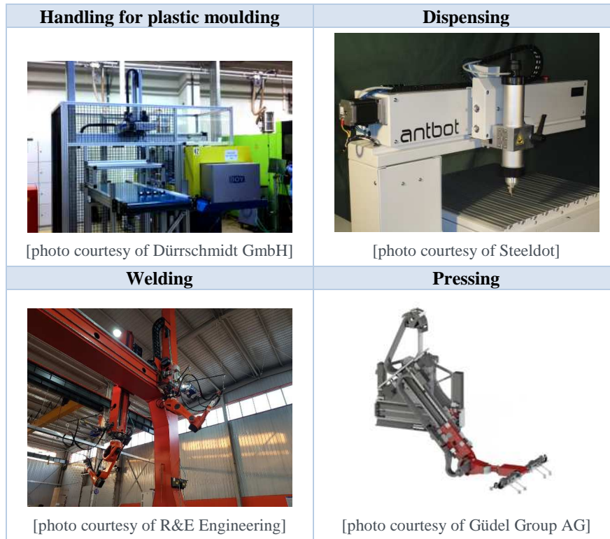
Figure 7.2-7 Examples of applications of Cartesian robots. Image rights: Dürrshmidt GmbH, Steel dot, R&E Engineering, Güdel Group AG.
